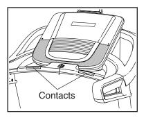
To measure your heart rate, stand on the foot rails and hold the pulse bar with your palms on the metal contacts; avoid moving your hands. When your pulse is detected, your heart rate will be shown. For the most accurate heart rate reading, continue to hold the contacts for about 15 seconds.
