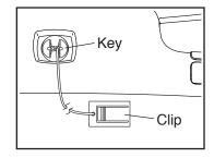
IMPORTANT: In an emergency, the key can be pulled from the console, causing the walking belt to slow to a stop. Test the clip by carefully taking a few steps backward; if the key is not pulled from the console, adjust the position of the clip.
