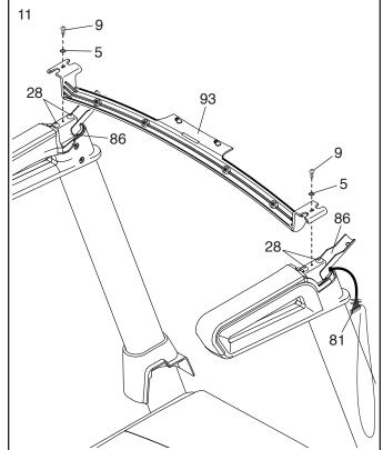
12. With the help of a second person, hold the console assembly (J) near the Handrails (86) (only one side is shown).
