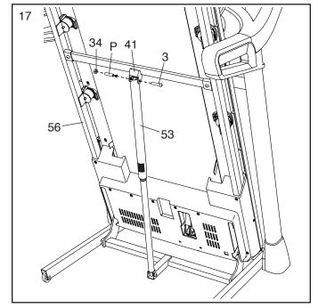
18. Firmly tighten the four 3/8" x 2 1/4" Screws (7), the two 3/8" x 1 3/4" Screws (62), and the two 3/8" x 1 1/4" Screws (63).
