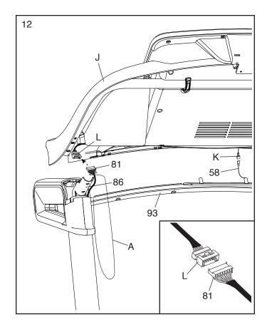
13. Set the console assembly (J) on the brackets on the Handrails (86). **Make sure not to pinch any wires.**
