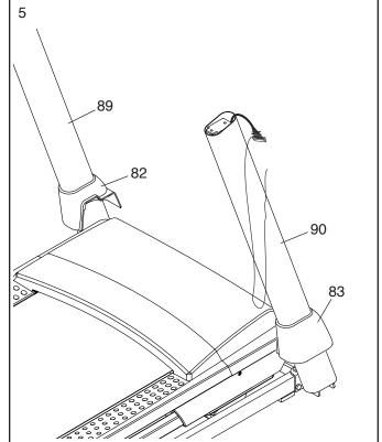
Identify the left handrail assembly (E). Attach the left handrail assembly to the Left Upright (89) with two 5/16" x 2 1/2" Screws (28) and two 5/16" Star Washers (11); do not fully tighten the Screws yet.
